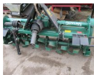
KILWORTH TRACTOR MOUNTED ROTAVATOR 1.8M
